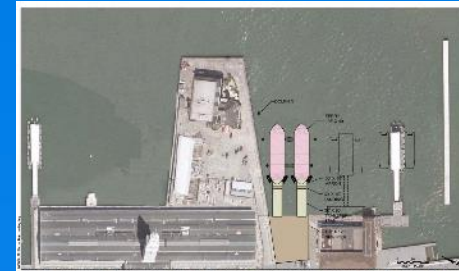
Figure 5.13 Gate E Bow Loading Concept: 699 pax Vessel (Source: Moffatt & Nichol May 2009)
