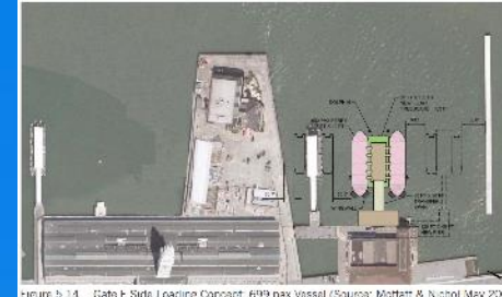
Figure 5.14 Gate F Side Loading Concept: 699 pax Vessel (Source: Moffatt & Nichol May 2009)
